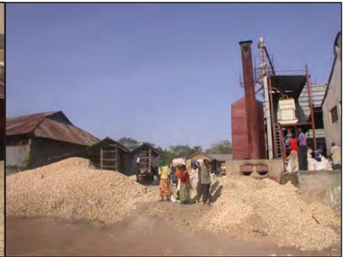
Recirculating dryer fuelled by shelled maize cobs.
